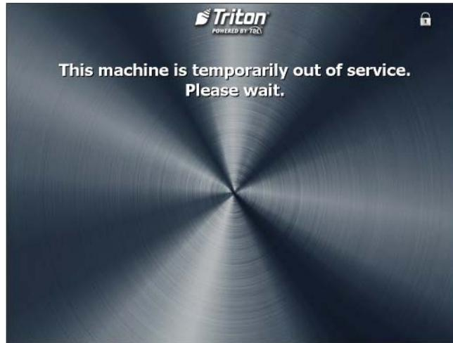
6. To clear the error, remove the metal from the reader. Wait until the ATM clears itself, approximate time of the "Metal Absent Time" value or wait until the screen displays "Card Reader Error. Error code: 196".
