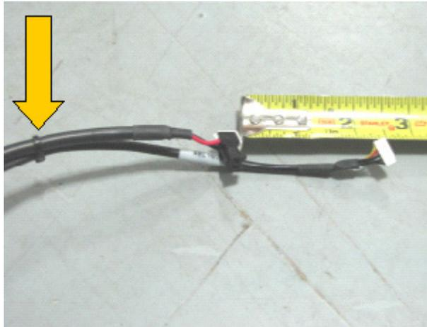
16. Pull the excess Data cable back up to the clips and make a “Bow”, *Left Image*. Place the excess cable into the clip, *Right Image*.
