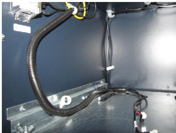
18. TY Wrap the end of the tubing by the clip. Trim excess TY Wrap, *Left Image*. TY Wrap the tubing at the opposite end. Trim excess TY Wrap, *Right Image*.
