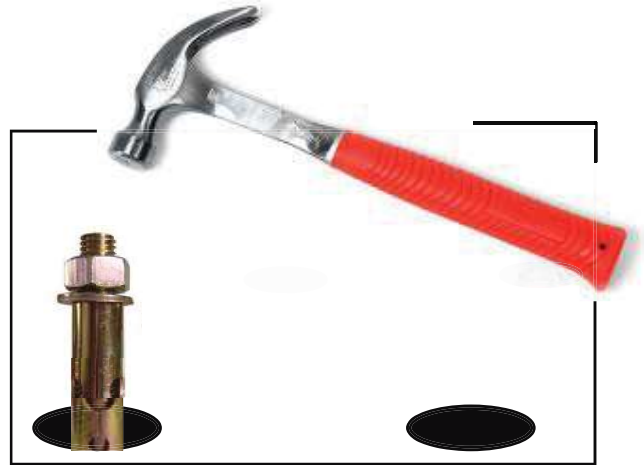
Hammer bolts snugly into drilled holes
