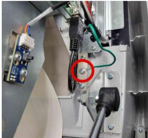
32. Insert the three screws connecting the ground wires.
