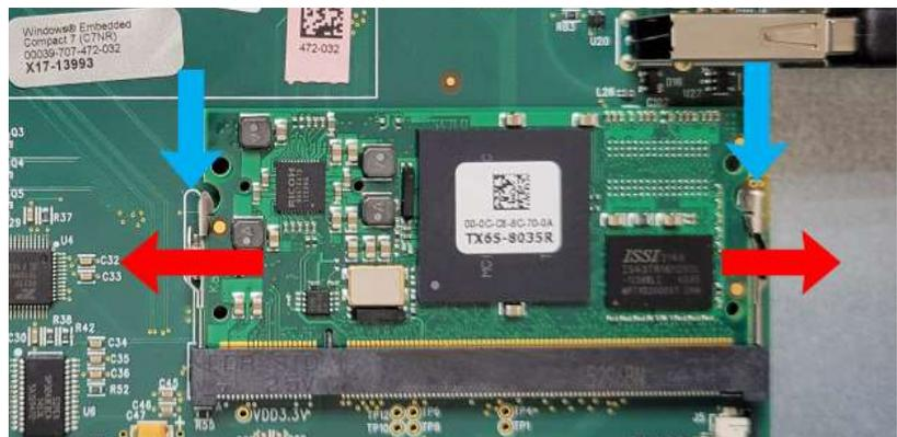
7. An **Incorrect** pull on the Module center-edge, **BLUE** arrow, may damage the memory components.
