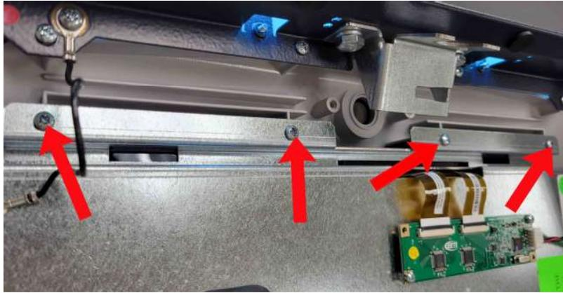
16. Remove and save 4 screws holding the display to the Control Panel.
