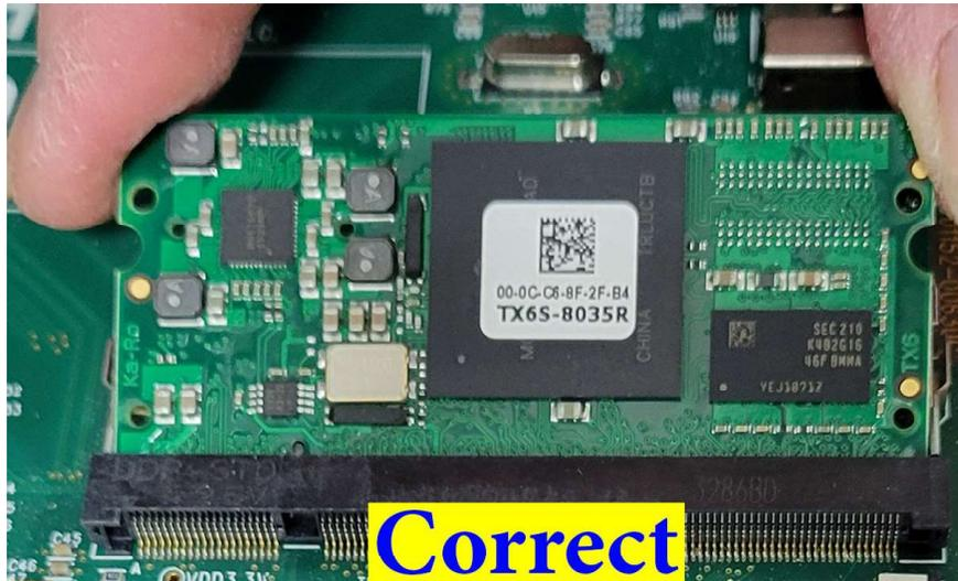
45. A **Correct** finger placement on the Module corners before pressing the Module into the clamps.
