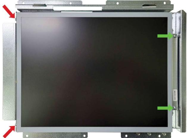
28. Obtain the front panel glass. On the *Left Image*, insert the ribbon cable through the bracket slot, **RED** arrows. Lower glass and center onto the display.
