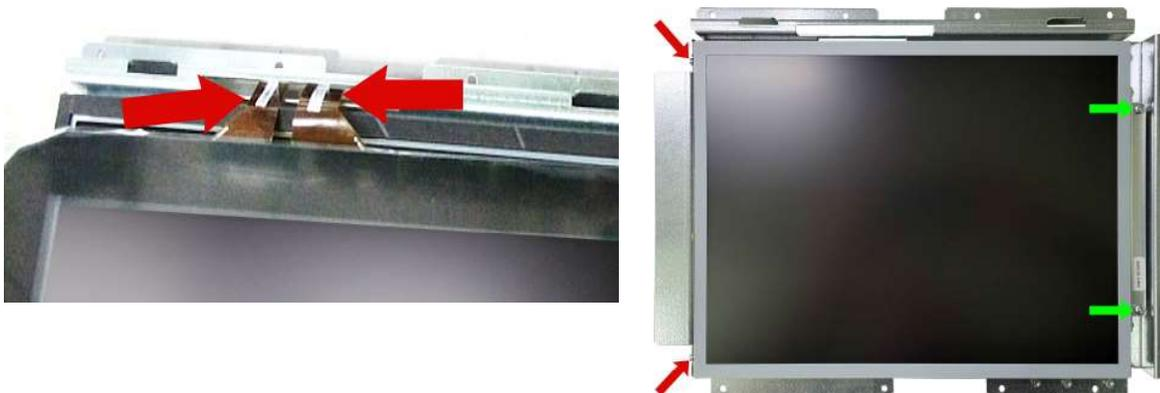
21. On the *Left Image*, turn display assembly face down. Lift bracket panel and pull the cable through the bracket opening. Place bracket aside for reinstallation. Lift one side of tape securing the cable to the back panel, **RED** arrows. DO NOT remove the tape from the back panel.
