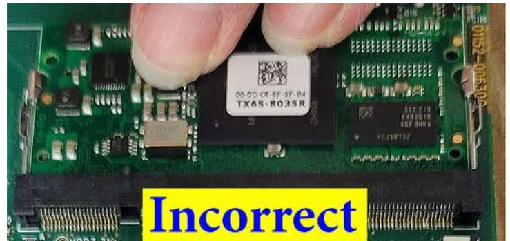
47. Visually inspect the Module is seated properly in the socket. The clamps, **RED** ovals, hold the Module in the socket. **ORANGE** arrows shows equal height of gold pins shown.
