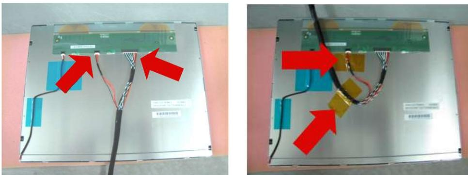
26. On the *Left Image*, insert the data cable through the display bracket opening, **YELLOW** arrow.
