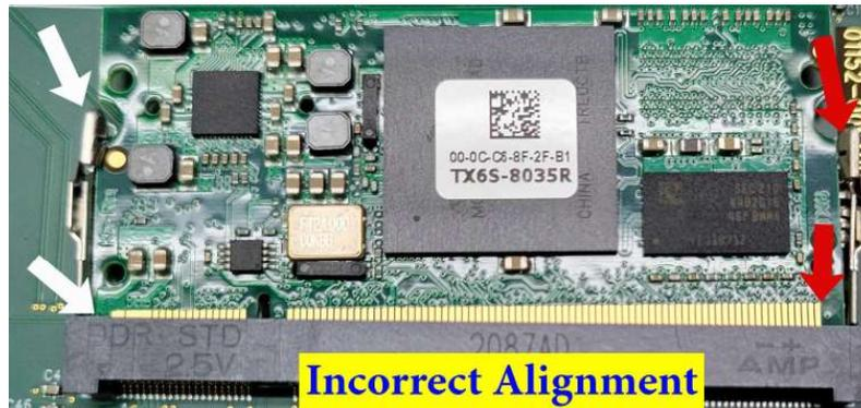
51. If the Module does not easily seat in the socket, remove the module and insert again.
