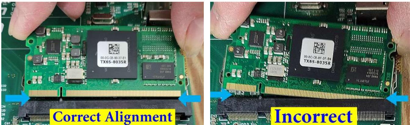
44. Hold the corners of the Module in **Correct** position and insert into the socket.
